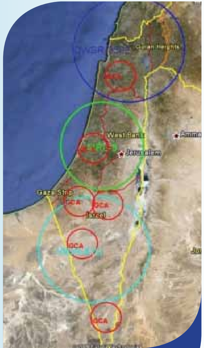
The 3 radars network covering bird movements across the entire airspace of Israel
