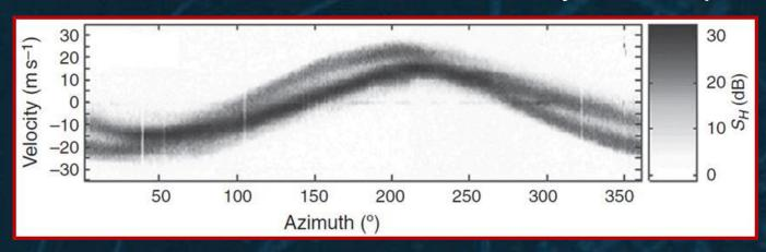
'Spectral VAD', showing two speeds – with slightly different directions.
