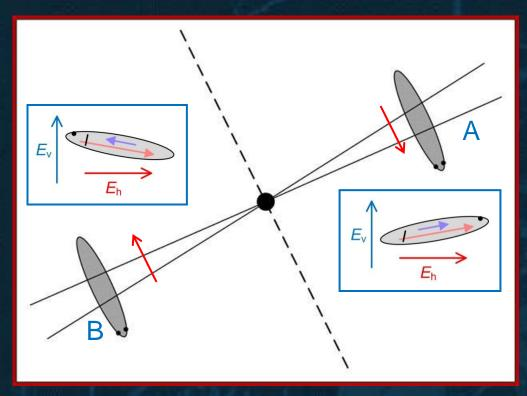
At A, H wave at phase when E is to right will induce a tail-to-head current.
