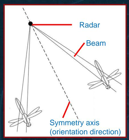
Insects have mirror symmetry. How can collectively oriented insects produce  $Z_{DR}$ ,  $\rho_{hv}$  and  $\phi_{DP}$  fields that are not mirror symmetric along the orientation direction?
