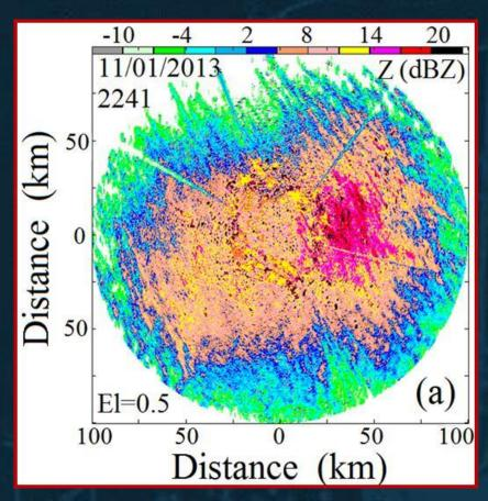
Z field shows some mirror symmetry, indicating collective orientation to SSE. Asymmetry may be due to different target densities to E and W.
