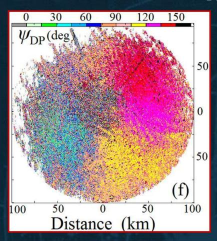
$\psi_{\text{DP}}$  ( $\approx \phi_{\text{DP}}$ ,  $\delta$ ) is again not density dependent, and its field again shows no mirror symmetry in the orientation direction.
