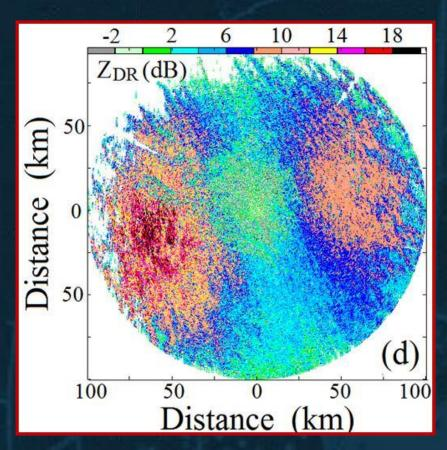
$Z_{\rm DR}$  is not density dependent. Its field shows mirror symmetry in the direction of collective orientation, but the symmetry is imperfect.
