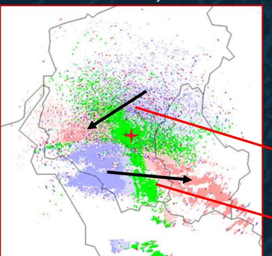
Birds and precipitation observed with C-band weather radar.
